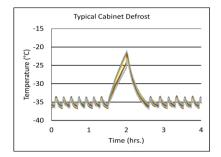
Performance data acquired at 22°C ambient, -35°C nominal set point in an empty cabinet with shelves using air probes, during stabilized steady state operation and a DAQ sampling rate of one measurement every 10 seconds
