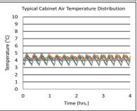
Performance data acquired at 22°C ambient, 4°C nominal set point in an empty cabinet with shelves using air probes, during stabilized steady state operation and a DAQ sampling rate of one measurement every 10 seconds
